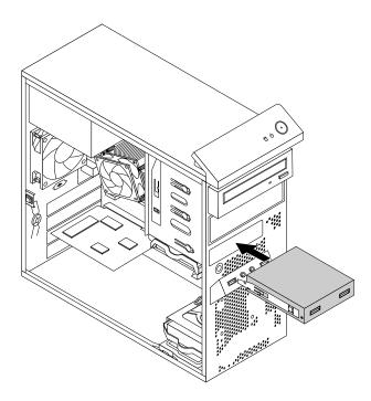
Figure 37. Installing the front USB assembly
