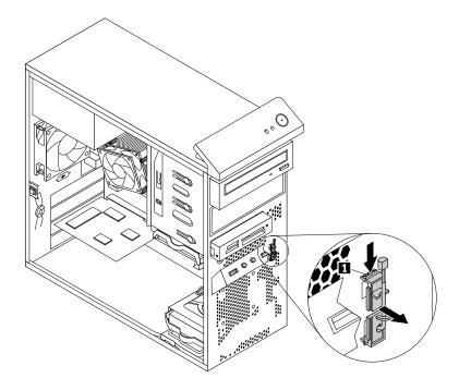
Figure 71. Removing the thermal sensor
