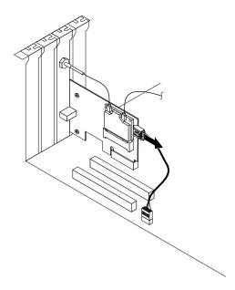
Figure 75. Disconnecting the Bluetooth cable
