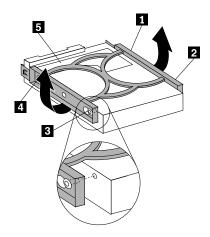
Figure 58. Installing the hard disk drive into the bracket
