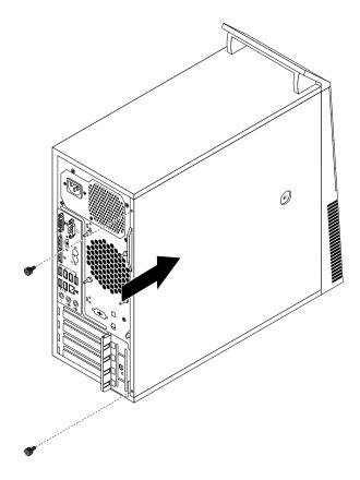
Figure 91. Reinstalling the computer cover
