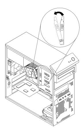
Figure 24. Removing the card reader retainer
