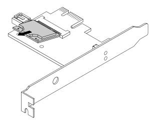
Figure 80. Removing the Wi-Fi card module
