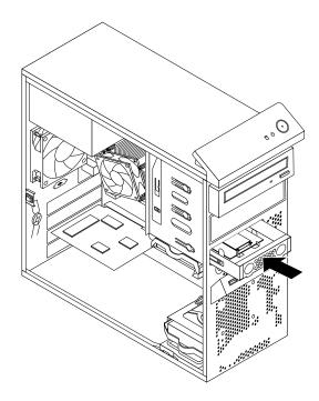
Figure 47. Installing the mSATA solid-state drive
