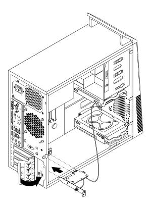
Figure 84. Installing the Wi-Fi adapter card
