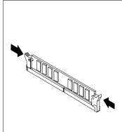
Figure 19. Installing a memory module
