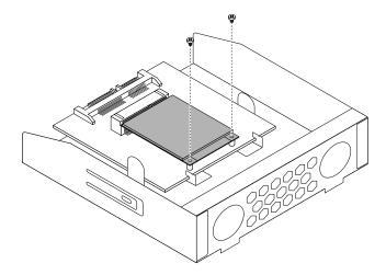
Figure 52. Installing the screws that secure the mSATA solid-state drive
