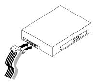
Figure 23. Connecting the optical drive
