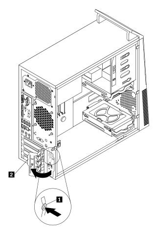
Figure 76. Opening the PCI card latch
