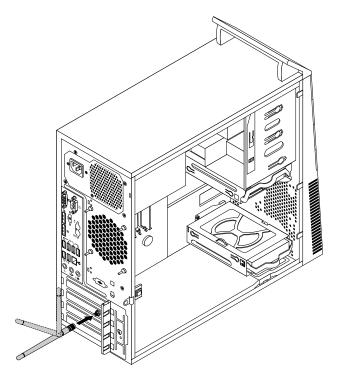
Figure 85. Installing the rear Wi-Fi antenna
