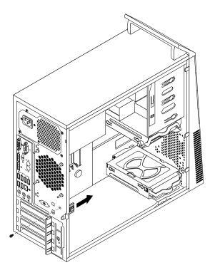
Figure 73. Removing the cover presence switch
