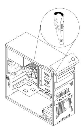
Figure 31. Removing the card reader retainer
