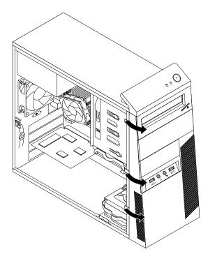
Figure 13. Removing the front bezel
