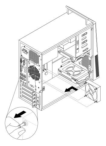
Figure 65. Installing the rear fan assembly
