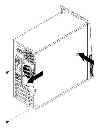
Figure 12. Removing the computer cover
