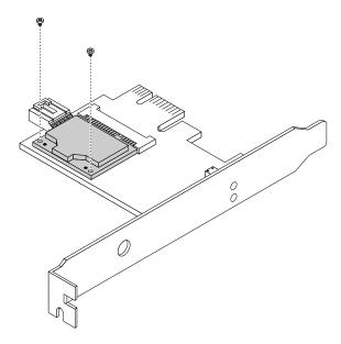
Figure 82. Installing the screws that secure the Wi-Fi card module
