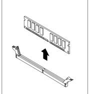
Figure 17. Removing a memory module
