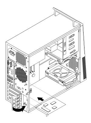
Figure 16. Installing a PCI card
