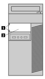
Figure 27. Removing the card reader cover
