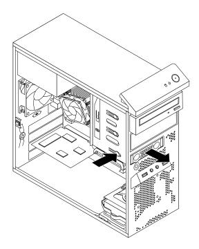
Figure 48. Removing the mSATA solid-state drive storage converter
