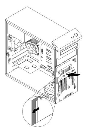
Figure 67. Installing the front audio and USB assembly
