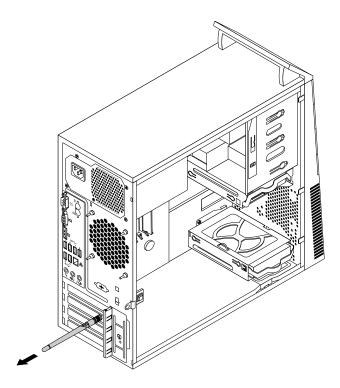
Figure 86. Removing the rear Wi-Fi antenna
