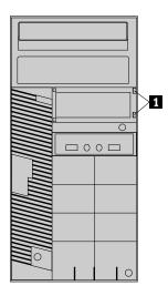
Figure 34. Removing the card reader cover
