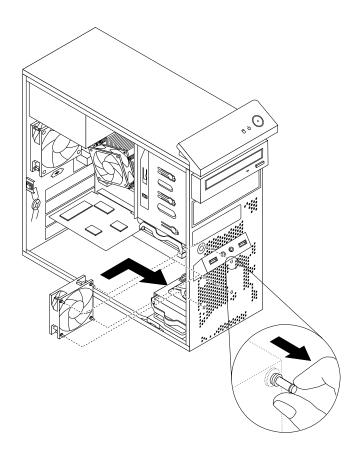
Figure 63. Installing the front fan assembly
