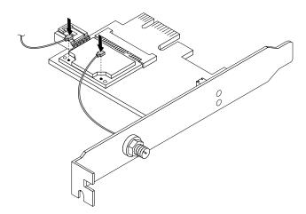
Figure 83. Installing the Wi-Fi antenna cables
