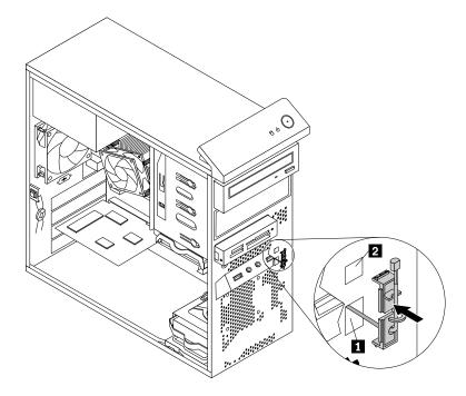
Figure 72. Installing the new thermal sensor
