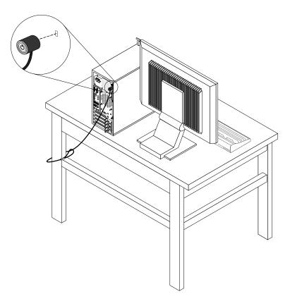
Figure 10. Attaching a Kensington-style cable lock
