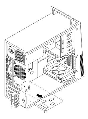
Figure 15. Removing a PCI card
