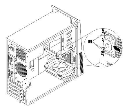
Figure 70. Installing a new internal speaker
