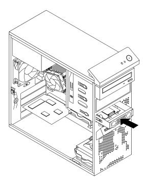
Figure 53. Installing the mSATA solid-state drive
