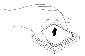
Figure 43. Removing the microprocessor
