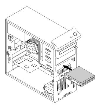
Figure 30. Installing the card reader
