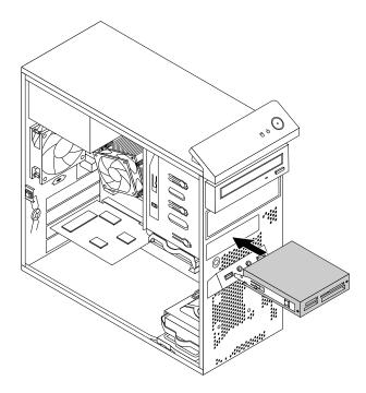
Figure 26. Installing the card reader
