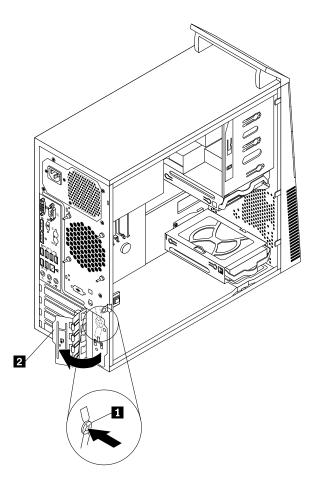
Figure 14. Opening the PCI card latch
