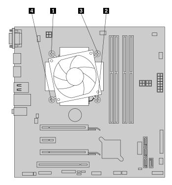
Figure 41. Removing the heat sink and fan assembly
