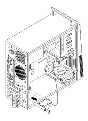
Figure 77. Removing the Wi-Fi adapter card
