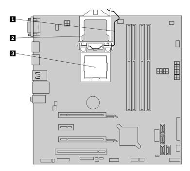
Figure 42. Accessing the microprocessor
