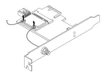
Figure 78. Removing the Wi-Fi antenna cables
