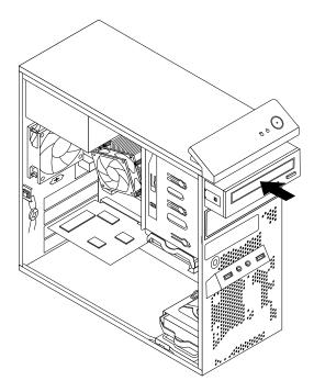
Figure 22. Installing the optical drive
