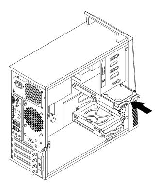
Figure 56. Installing the primary hard disk drive
