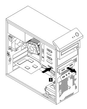
Figure 35. Removing the front USB assembly
