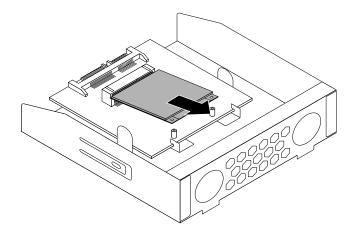
Figure 50. Removing the mSATA solid-state drive
