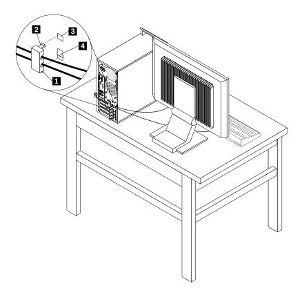
Figure 11. Attaching a cable lock
