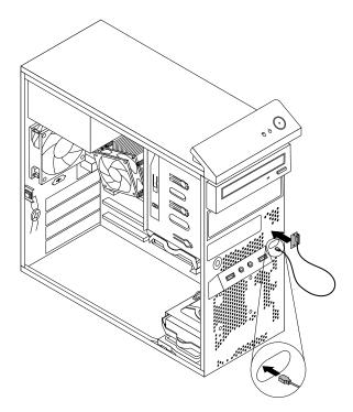
Figure 88. Installing the front Wi-Fi antenna
