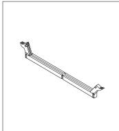
Figure 18. Opening the retaining clips
