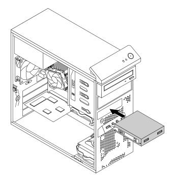
Figure 33. Installing the front USB assembly
