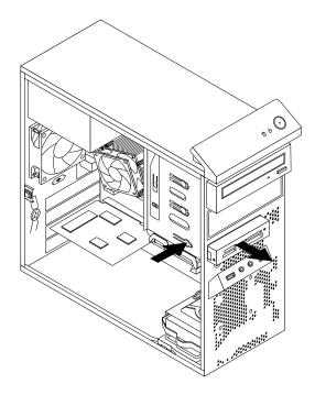
Figure 28. Removing the card reader
