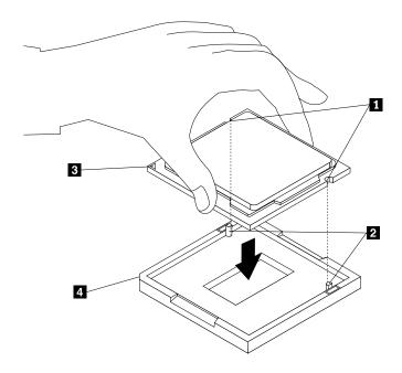
Figure 44. Installing the microprocessor
