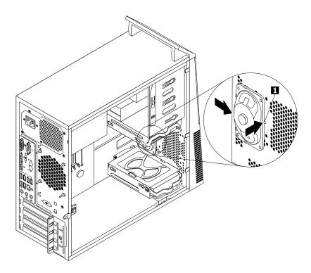
Figure 69. Removing the old internal speaker
