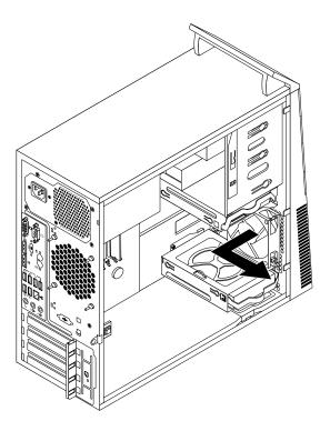
Figure 62. Removing the front fan assembly
