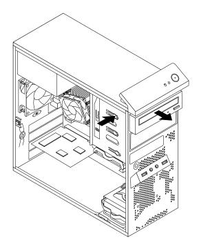
Figure 20. Removing the optical drive
