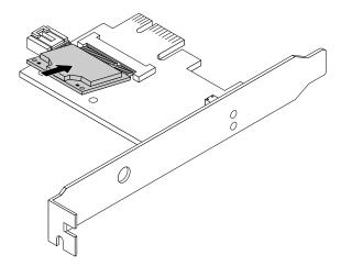
Figure 81. Installing the Wi-Fi card module
