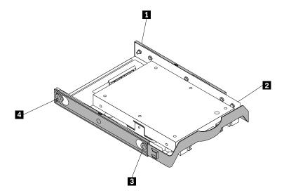
Figure 61. Installing the solid-state drive with the storage converter into the hard disk drive bracket
