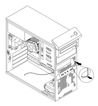
Figure 89. Removing the front Wi-Fi antenna
