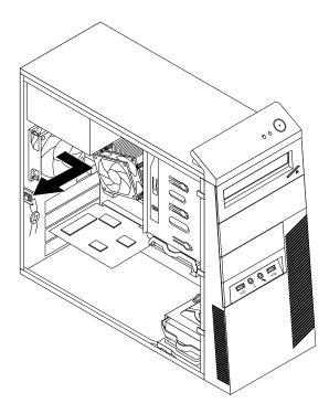
Figure 64. Removing the rear fan assembly
