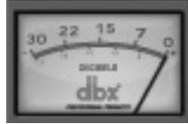
Indicates the amount of gain reduction being applied. Click to open or close the Dynamics Control Panel (described on page 13).
