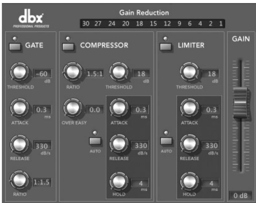
Inputs 1-8 in the Mixer feature Channel Strip Dynamics, including a gate, compressor, limiter, and a gain fader. To open the Channel Strip Dynamics, click the Gain Reduction meter/button at the top of the channel's "strip" in the Mixer.
