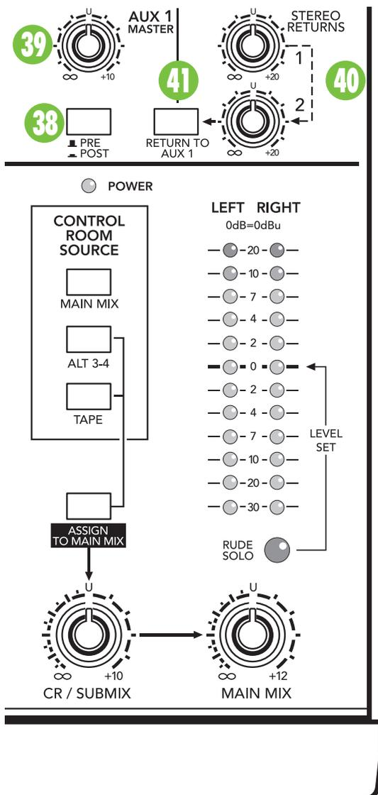
These outputs can be fed to the inputs of a reverb or other device. From there, the outputs of this external device are fed back to the mixer’s stereo return [7] jacks, then these signals are sent through the stereo return [40] level controls, and finally delivered to the main mix.
