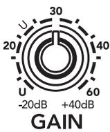
Gain adjusts the input sensitivity of the mic and line inputs connected to channels 1 through 4. This allows signals from the outside world to be adjusted to optimal internal operating levels.
