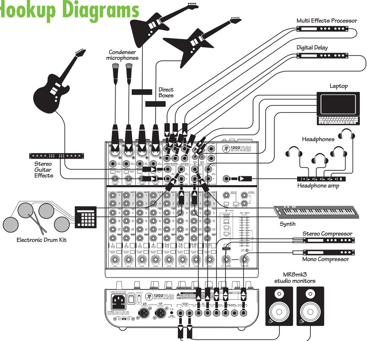
This diagram shows microphones connected to the mic inputs of channels 1 and 2, and a vocal compressor connected to the channel 1 insert jack. Bass and electric guitars are attached to channels 3 and 4 via DI boxes with a stereo compressor on the insert. The lead guitar plays through a stereo effects processor plugged into channels 5 and 6. An electronic drum kit is connected to channels 7 and 8, while a synth is connected to the line inputs of channels 9 and 10.
