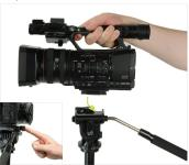
10 Mount the Camera to the Tripod
