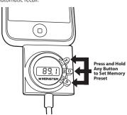
NOTE: After using AutoScan 3D, the selected frequency will automatically be stored to the "S" button's memory for instant recall.
