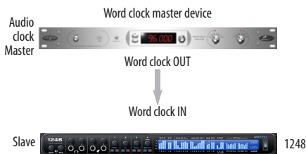
Figure 4-12: Slaving your MOTU device (a 1248 in this example) to word clock. For the 1248 clock source, choose ‘Word Clock In’.
