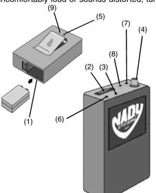
(9) on the back of the receiver counter-clockwise until good audio quality is obtained. If volume is too low, turn the AUDIO LEVEL CONTROL (9) clockwise until you obtain comfortable volume.
