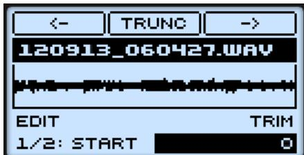
The EDIT page on the controller, page 1 of 3: adjusting the start and end point of the Sample.
