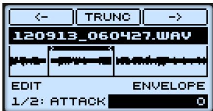
The EDIT page on the controller, page 3 of 3: setting the amplitude envelope of a Sample.
