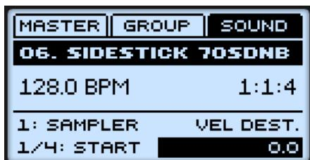
Sampler parameters – page 6 of 6 on the controller.
