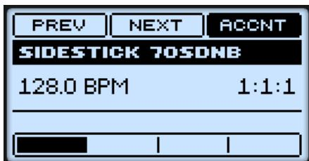
The Step mode on the controller: the first bar of a four-bar Pattern.
