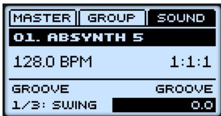
The Sound's Groove Properties on the controller.
