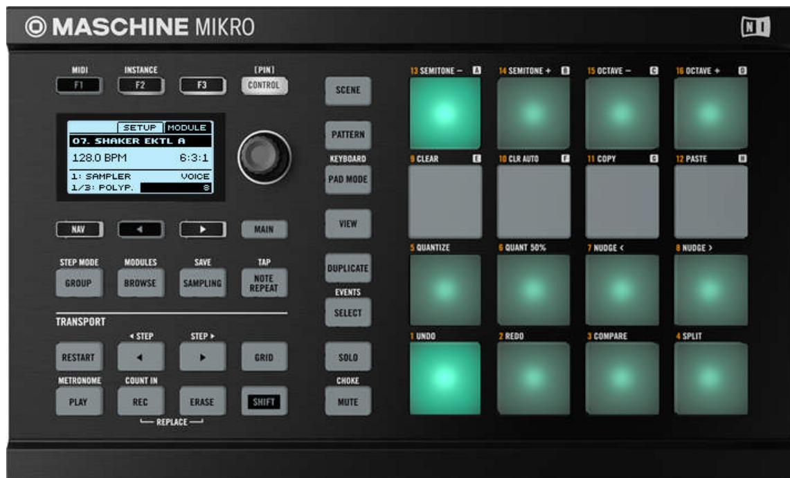
Shortcuts for navigating the Module slots from the MASCHINE MIKRO controller while holding NAV.
