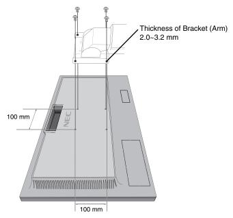
Weight of LCD assembly: 2.9 kg (E203Wi) 3.7 kg (E233WM)
