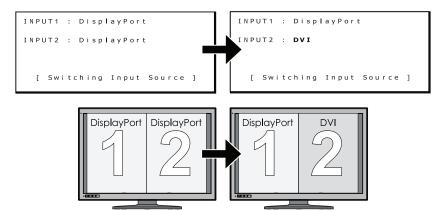
**NOTE:** Using INPUT 1 and INPUT 2 with different input sources (DVI + DisplayPort) is not recommended for standard applications. It may result in slight differences of luminance and color between left and right screen and/or a frame skip (See page 9).
