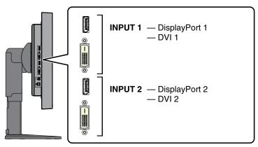
Input ports are located on the side of the display.
