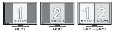
The following shows an example of the case when the resolution of 3072 x 2048 is selected for INPUT 1 and QXGA (1536 x 2048) is selected for INPUT 2.
