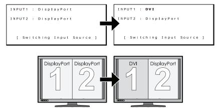
Press the plus (+) button on the front bezel without displaying the OSD menu and the input source of INPUT 2 is switched.
