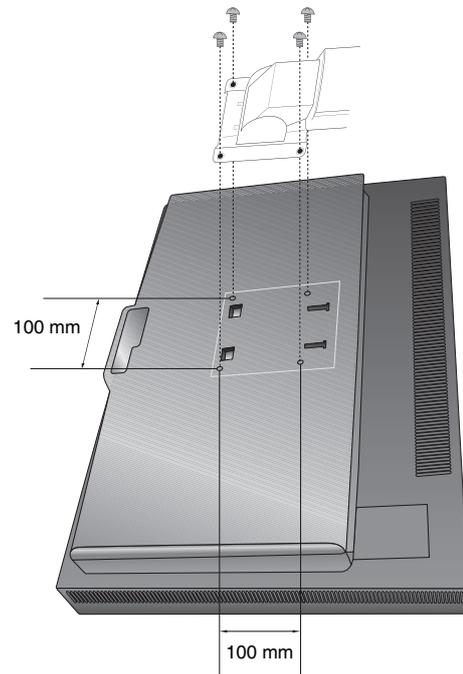
Weight of LCD assembly: 4.8 kg
