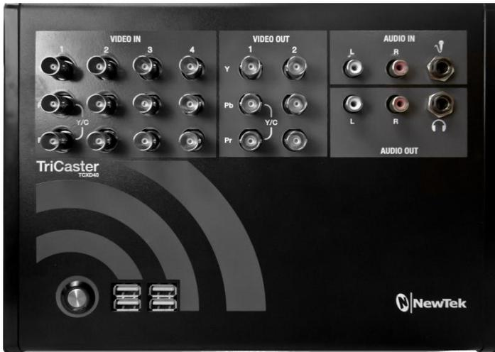
TriCaster lets you ‘live switch’ up to four HD (or SD) cameras or other analog inputs, along with internal and network connected sources. You can even mix SD and HD sources. In addition, multiple external audio sources can be added to your program.
