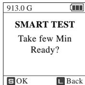
The Smart Test takes several minutes to test the internal hard drive. Pressing the control key initiates the Smart Test.
