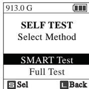
The User can choose either a Smart Test or a Full Test. Choose the Smart Test. The Smart Test uses an S.M.A.R.T test provided by the hard drive.
