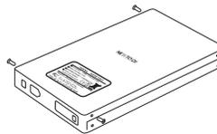
Put the cover on again. Make sure to observe the correct orientation. The larger foam part on the inside of the cover should face in the direction of the power socket/USB port.
