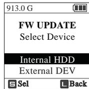
The firmware file (NEXTOMS.BIN) should be placed in the root directory of a memory card or the internal hard drive. Select [In HDD] (hard disk drive) if the firmware file is to be placed in the root directory of the internal hard drive. Select [In Memory Card] if the firmware is in the root directory of the memory card. If you selected the memory card, insert the memory card into the ND2901.
