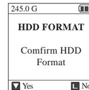
Then you can repartition and reformat the internal hard drive; to confirm, push the control key downward. All data on the internal hard drive will be lost!
