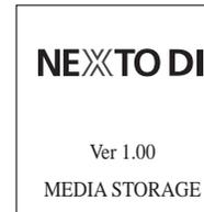
Press the control key for more than 2 seconds in order to turn the ND2901 on. The power up logo and firmware version is shown on the LCD. When you see the logo on the LCD screen, release the button. Otherwise, the ND2901 will automatically power down.
