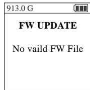
If a valid firmware file is not contained in the specified device, the ND2901 indicates an error. Check whether the device contains valid firmware in the root directory and repeat the previous process.
