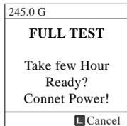
The Full Test will take several hours. So you need to connect power to the ND2901. It will read all the sectors in the internal hard drive to discover if any bad sectors exist.
