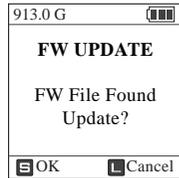
If valid firmware is found at the specified location, the ND2901 indicates a "FW File Found" message on the LCD. Confirm the firmware upgrade by pressing the control key briefly S.
