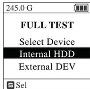
The user can choose either an internal hard drive or an external hard drive, or a memory card.
