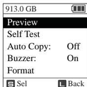
Press the control key once at the "XCopy Ready" mode to activate the menu.
