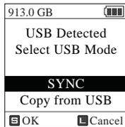
If the proper external USB hard drive is connected, the ND2901 shows “SYNC” or “Copy from USB” mode selection. Briefly press the control key to select ‘SYNC’.
