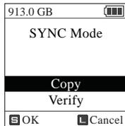
A user can select two modes of duplication, copy or verify. Highlight the desired mode using the up/down key, then briefly press to select the mode. Press and hold the key **[L]** to cancel the operation.
