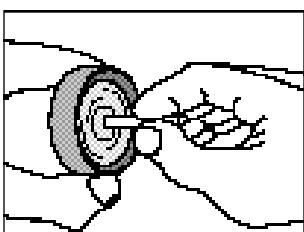
Starting in the center of the lens, gently rub in a circular motion from the center to the outside.
