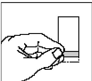
Roll the tissue into a cylinder and moisten only one tip with lens cleaning fluid.
