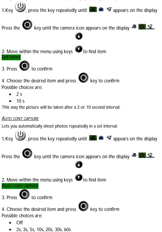
Press the shutter key (down arrow) to take a picture according to the set interval of seconds. Press the shutter key again twice to stop the sequence.
