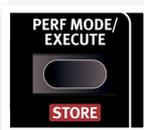
To switch between these modes, press the Perf Mode button repeatedly. When the LED displays a two or three digit number between 1.1 and 4.99, then the Program Mode is active. Performance Mode is indicated by the initial letter P, followed by a number from 1 to 99.
