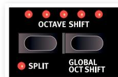
The center LED indicates when no octave shift is applied.
