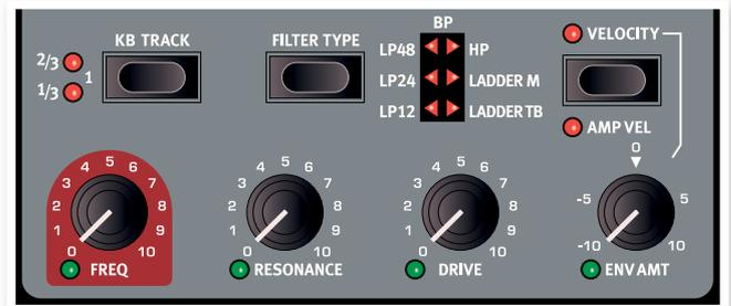
The Filter is one of the most important components to create the overall timbre of the sound. The harmonic content that the oscillators produce can be shaped with the filter and the filter itself can be modulated with various functions. The Nord Lead 4 features a selection of traditional synthesizer low pass, band pass and high pass filters, a steep 48 dB low pass filter and two unique emulations of filters that we have modeled from two vintage synthesizers, the Ladder M and the Ladder TB.
