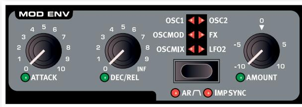
The Modulation Envelope is an envelope with Attack, Decay/Release and Amount controls. It can be used to modulate various destinations in the Nord Lead 4 and will normally be triggered when you press a key, just like the Amp and Filter envelopes. The modulation from the envelope can be both positive or negative, this is determined with the Mod Env Amount knob.
