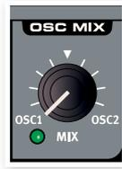
Most of the knobs have a green LED indicator below them. This LED is used for indicating when a parameter is connected to a Morph source. Please refer to page 13 for more information on morphing.
