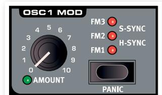
There are two types of Oscillator Modulation available: Frequency Modulation and Oscillator Sync.
