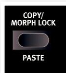
You can also copy a complete Morph setting, or an entire Slot. Hold Copy and press a Morph, Slot or Impulse button. "Cpy" will be displayed in the LED.
