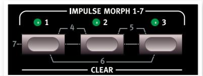
closed filter in the program, and have an Impulse Morph open up the filter when you press the Impulse button. By combining two or all three buttons, you have a total of 7 Impulses available for each program.
