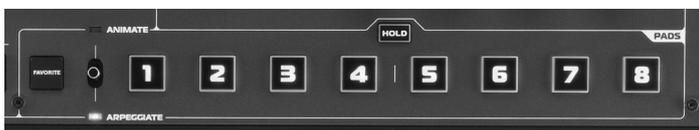
Arpeggiator operation in the MiniNova is controlled by the three **ARP** buttons [19], [20] & [21]: **ON**, **LATCH** and **TEMPO**. The **ON** button enables or disables the Arpeggiator.
