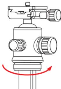
Remove the screw, and insert the opposite end back into the plate. Mount the plate back onto the tripod by turning it clockwise. To mount a head, align the bottom of the tripod mount with the tripod's mounting screw, then twist clockwise until fully secured. Do not over-tighten, as this may cause damage.
