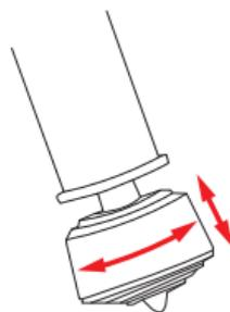
*\*Model CC-2441 features a removable rubber cap with a spike beneath it on each tripod leg. To exchange a rubber foot for a spiked foot, simply pull the rubber cap off the leg, exposing the spike underneath. When a rubber foot is desired, replace the rubber cap over the spike.*
