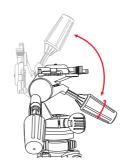
Turn the knob counter-clockwise to unlock and clockwise to lock it. After positioning the head, make sure to securely tighten the knob.
