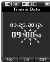
You can select between 12 and 24 hour display by pressing the **F2 (24H)** button while setting the hour and minute.
