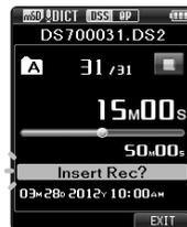
**2** While playing the file, press the **F1 (INSERT)** button to insert an additional recording.
