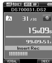
**4** Move the slide switch to the **STOP (■)** position to stop inserting the additional recording.
