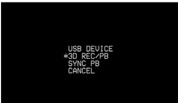
**3** Use the Up/Down cursor buttons to place a "\*" next to 3D REC/PB, and press the **SET** button.
