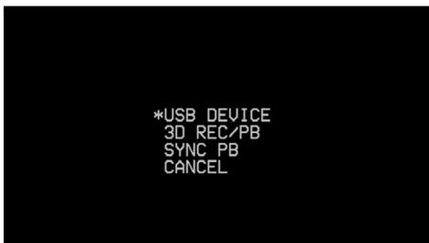
“USB DEVICE” flashes on the LCD monitor to indicate that the unit is entering the USB host mode. After the mode switch, “USB DEVICE DISCONNECT” appears on the LCD monitor.
