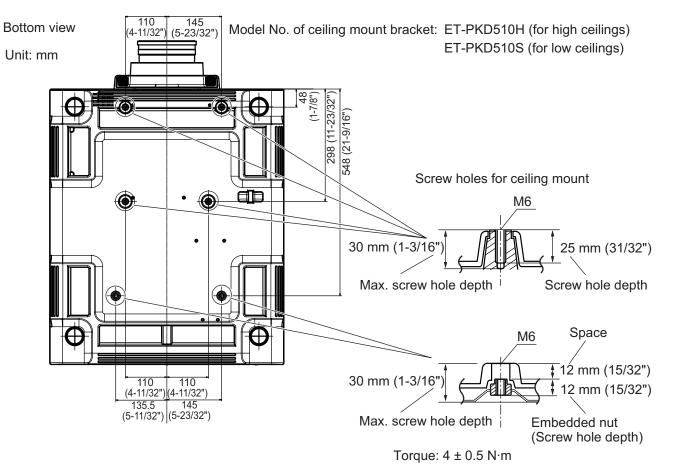
• Make a clearance of at least 5 mm (0.2") between the projector bottom and setting surface by inserting spacers (metallic) etc. between them.
