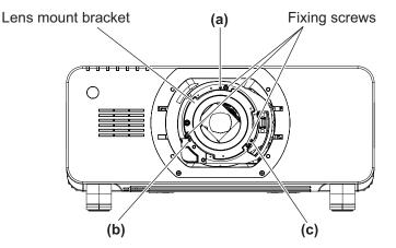
(Focus adjustment screws (a), (b), and (c) are adjusted with the lens attached.)
