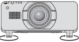
Adjustable range Front adjustable feet: 12 mm (15/32") Rear adjustable feet: 12 mm (15/32")
