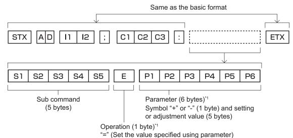
\*1: When transmitting a command which does not need a parameter, the operation (E) and parameter are not necessary.
