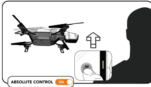
When absolute control is enabled, with you facing the AR.Drone 2.0 (**Joypad mode** enabled):
