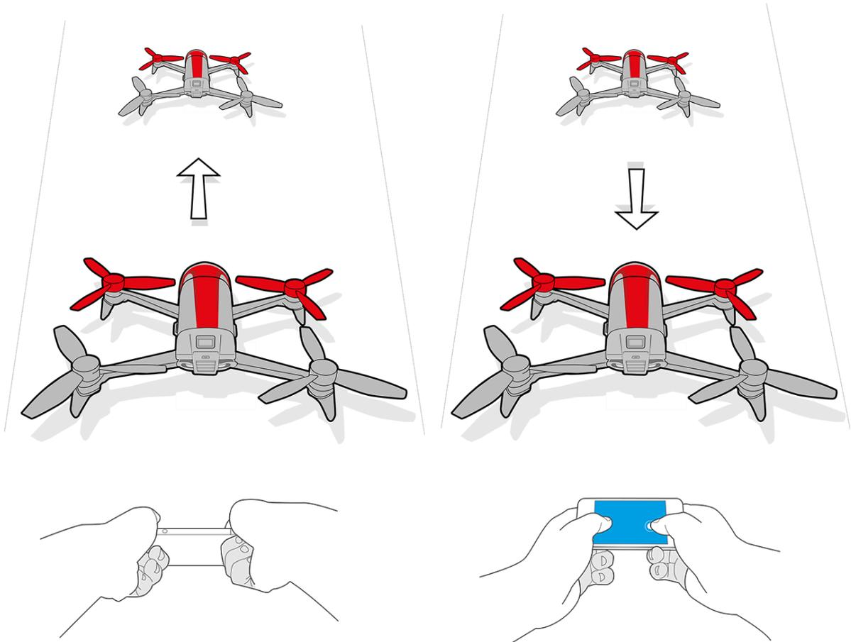
*Hold the central button and tilt your smartphone forwards or backwards to pilot the Bebop 2 forwards or backwards.*
