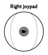
Slide to orientate the camera regardless of the Parrot Bebop Drone's position.
