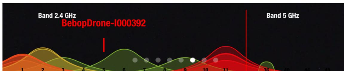
Red curves represent congested channels. Green curves represent less congested channels. The channel without curves are free.
