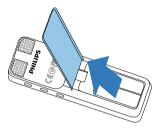
Insert the batteries or rechargeable batteries into the device as shown. Ensure correct polarity!
