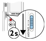
2 To power off, pull down the power switch on the side of the device again and hold for about two seconds.
