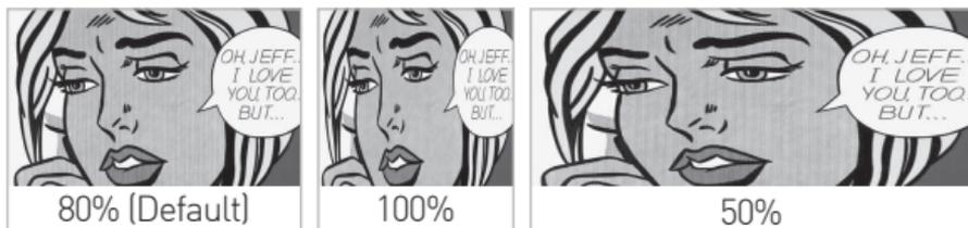
The appearance of your image in frame is affected not only by the speed of pixelstick, but the speed at which you move pixelstick. Below is an example of how the speed setting affects an image, given that the user is moving at a similar rate.
