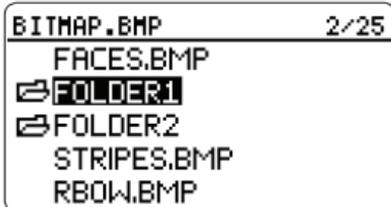
Press FIRE. The backlight will turn off and the image will display. When finished, pixelstick will return to the Main Menu with the backlight off until a key press. Pressing FIRE a second time before completion will cancel.
