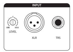
Line-level Inputs. The Sceptre S6/S8 provides a choice of two balanced inputs: XLR and ¼"TRS. These inputs accept a line-level signal from your audio source and feed that signal to the monitor's built-in power amplifiers. When both balanced connections are in use, the TRS input supersedes the XLR input.
