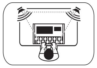
The speakers should be separated so that the coaxial drivers form an equilateral triangle with your head. The monitors should be "toed in," or angled, so that they are pointed at you, not pointed straight ahead.
