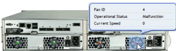
When a power supply fan fails, you must replace the power supply. See “Replacing a Power Supply” on page 323 for more information.
