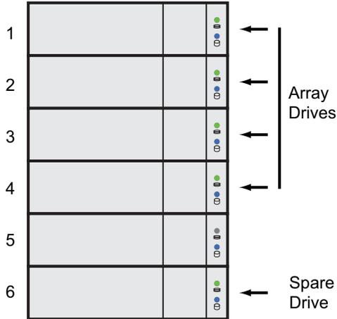
In the example above, there is a four-drive RAID 5 disk array and a global spare drive. Physical drives 1, 2, 3, and 4 belong to the disk array. Physical drive 5 remains unconfigured. Physical drive 6 is a revertible spare drive.
