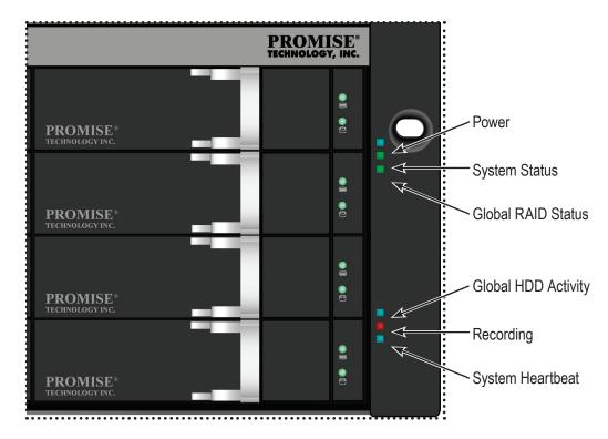
Vess A2600/A2600s Front Panel LEDs - Right side
