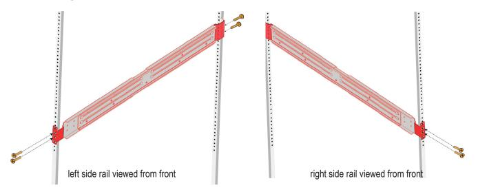
Place enclosure into the mounting rails
