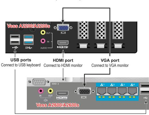
USB, HDMI and VGA interfaces on rear panel
