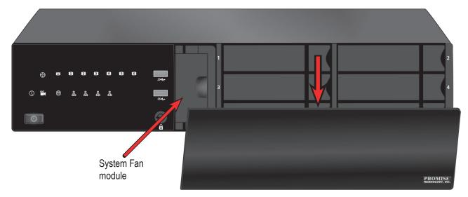
With the cover removed, you can access the System Fan module from the front.
