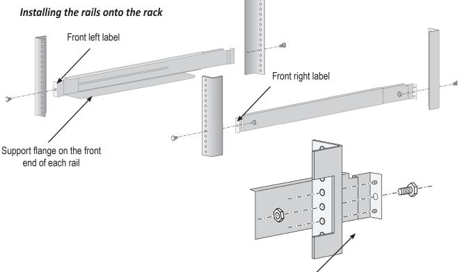
Guide pins on rails align with holes in the rack post
