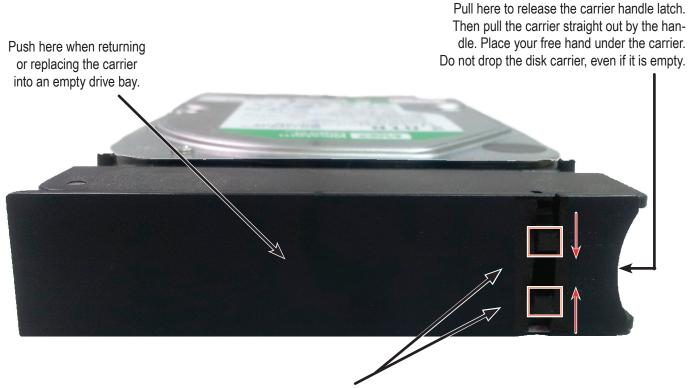
Tabs for locking mechanism insert. This piece must be removed to unlatch the carrier. To remove, squeeze the tabs together and pull out. To reinsert, squeeze the tabs together and replace in position. Do not discard the locking mechanisms.
