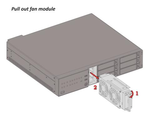
To replace the fan, repeat the same steps in the reverse order. Slide the module straight into the open module space so that it is firmly seated, then swing the handle back into place so it is flush with the front of the module.
