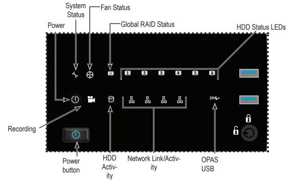
Front panel LED behavior for Vess A2200/A2200s system:
