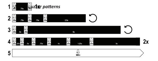
Other alarm patterns include three short buzzes followed by a longer silence, then repeated (example number 2 above). This can indicate a serious problem that requires immediate action such as high enclosure temperature or the system fan is not installed. If you hear this, check the System Status and Fan LEDs. If these are normal, it might indicate a physical drive problem, or a power supply problem. Check the event log for more information.
