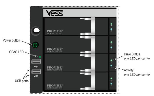
Vess A2600/A2600s Front Panel LEDs - Left side
