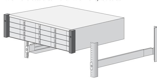
3. Secure the VTrak subsystem to the rack.
