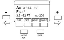
The Fill setting is used to adjust the flash output from 3 stops (-3) below the camera setting to 2 stops (+2) above the camera setting. The Fill can be adjusted in 1/3 steps.
