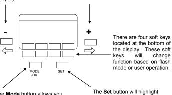
The **Mode** button allows you to change the mode of the Trio. Pushing it will bring up the mode change menu.
