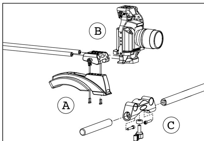
A: Attach Shoulder Pad to Rod Clamp using provided screws.
