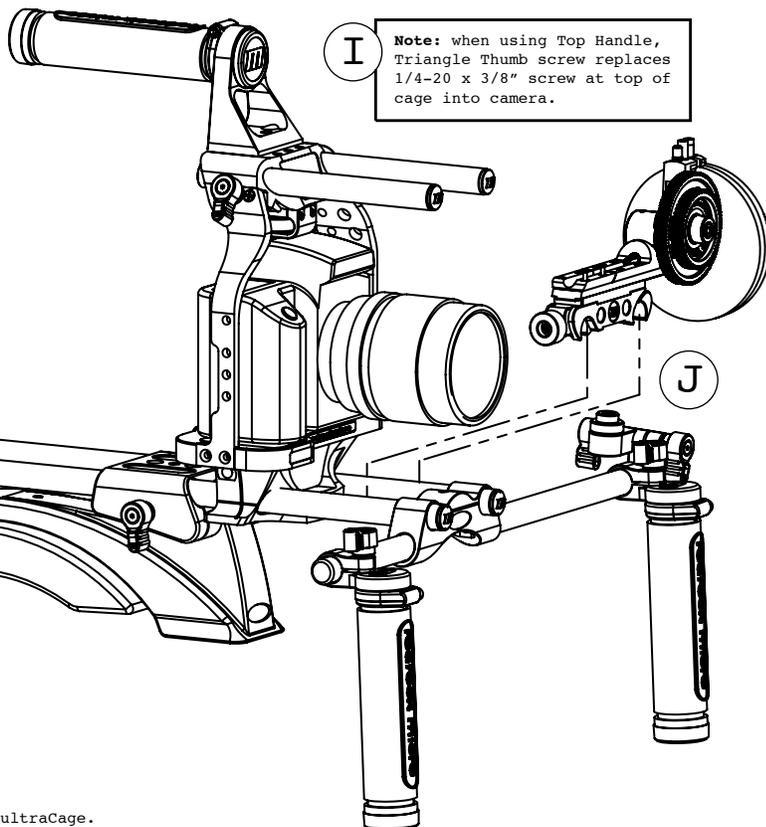
I Note: when using Top Handle, Triangle Thumb screw replaces 1/4-20 x 3/8" screw at top of cage into camera.
