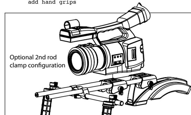
Deluxe Bundle Configuration Option 2: Attach camera to 2nd rod clamp. This configuration allows you to use the onboard LCD on your camera. (2nd Rod Clamp sold separately)
