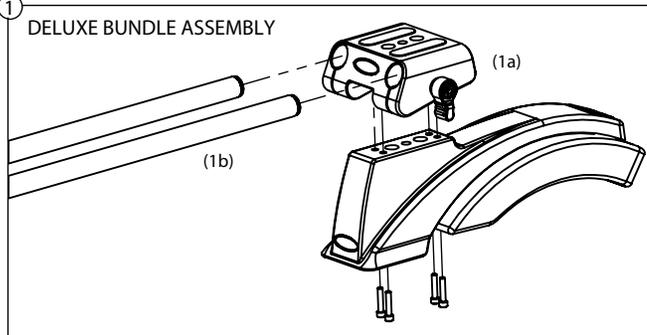
(1a) Attach rod clamp to shoulderPad
