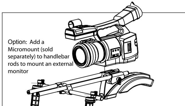
Deluxe Bundle Configuration Option 1: Attach camera to rod clamp / shoulderPad assembly using camera screw
