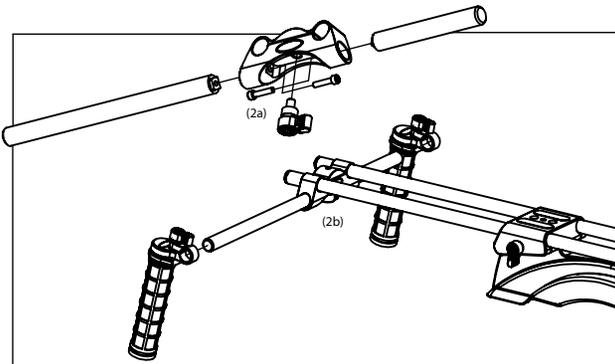
(2a) Attach rods to rigid mount using screws
