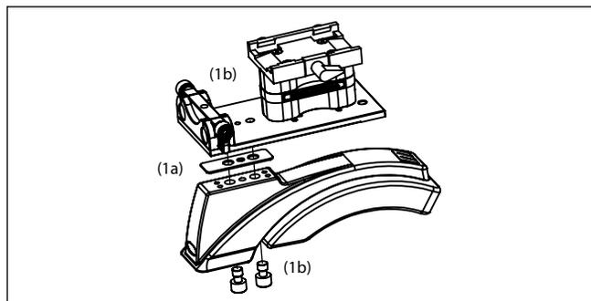
(1a) Add adhesive pad to top of shoulder pad (this is the rubber one with three holes for the threads)
