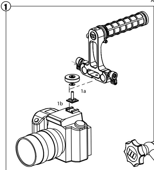
(1a) Attach microshoe attachment to microHandle by threading the shoe part through the bottom of the handle. Once shoe is in place, attach washer and screw to complete assembly
