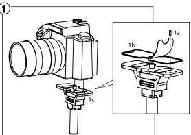
(1a) Attach camera specific set screw to DSLR Baseplate. Kit comes with Canon and Nikon set screws
