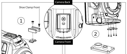
Position Shoe Clamp in camera shoe mount 2: Remove standard mounting plate from as shown and tighten screw. Note: Shoe Clamp MUST be placed so the free 1/4-20" mounting hole is nearest
