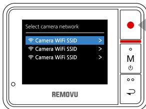
1. Turn on your HERO4 camera and go to HERO4 Setup → RC & App → Select Existing to turn on the Wi-Fi function.
