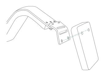
4 Attach the counterweight by threading the remaining two screws through the mounting plate and into the counterweight. Use the hex key to fasten the screws until fully tightened.
