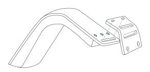
Attach the mounting plate by threading two of the included hex screws through the slot and into the screw holes. Use the included hex key to fasten the screws until fully tightened.
