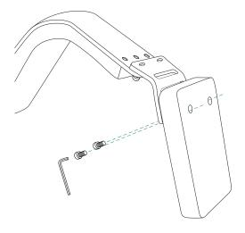
Important: The screws should go easily into the holes of the counterweight. If you feel resistance when turning the screws, turn the counterweight over and repeat the previous instruction.
