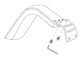
Align the counterweight's screw holes with the corresponding screw holes on the outside of the mounting plate.
