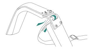
Adjust the length of the back strap by placing the SR-1000 rig on your shoulder. The strap should be a maximum of 6 inches above your waist.
