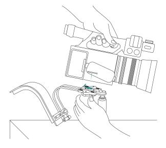
With the SR-1000 support rig and camera on the secure surface, attach the back strap to the back of the waist strap with the quick release and move the sliding lock to the locked position.
