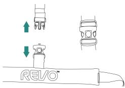
Adjust the waist strap so that it fits snuggly. The logo on the waist strap should face out with the air mesh facing towards you. Attach the quick release and move the sliding lock to the locked position. Keep the strap attached around your waist while you complete the rest of the steps.
