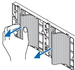
(2) Push the left edges of the filters and remove the two hard honeycomb filters (large and small).
