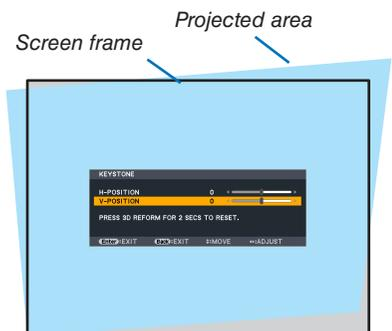
3. Align the left (or right) side of the screen with the left (or right) side of the projected image.
