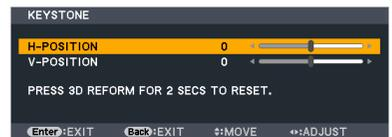
2. Press the ▼ button to select [V-POSITION] and then use the ◀ or ▶ so that the left and right sides of the projected image are parallel.
