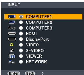
2. Press the ▼ or ▲ button to select [NETWORK] and press the Enter button.
