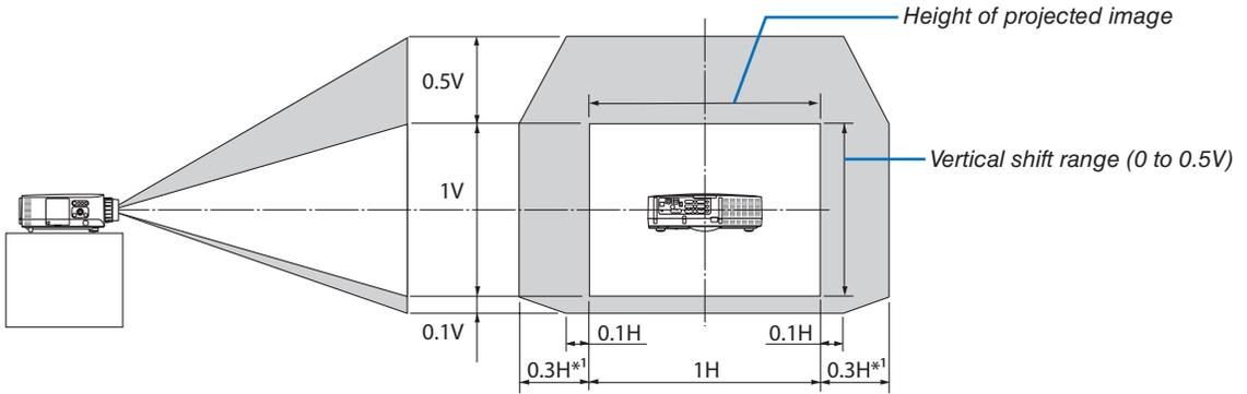
*NOTE\*1: Horizontal lens shift range is 0.15H at 150" projected image with the PJ Standard Lens Type1*
