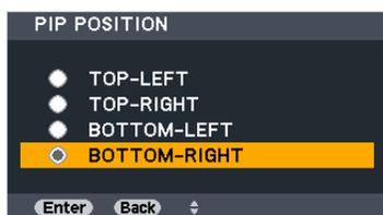
Use the ▲ or ▼ button to select the sub picture's position and press the Enter button. The options are: TOP-LEFT, TOP-RIGHT, BOTTOM-LEFT, and BOTTOM-RIGHT.
