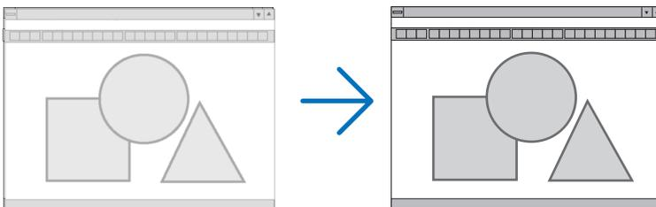
**PHASE** ..... Use this item to adjust the clock phase or to reduce video noise, dot interference or cross talk. (This is evident when part of your image appears to be shimmering.) Use [PHASE] only after the [FREQUENCY] is complete.
