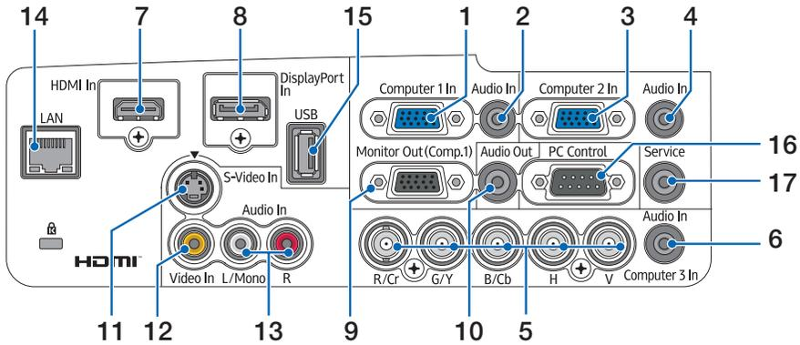
1. **Computer 1 In/ Component Input Connector (Mini D-Sub 15 Pin)** (→ page 13, 140, 145)
