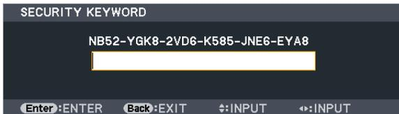
3. Type in the correct keyword and press the Enter button. The projector will display an image.
