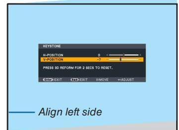
4. Press the ▲ button to select [H-POSITION] and then use the ◀ or ▶ so that the top and bottom sides of the projected image are parallel.
