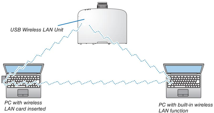
To enable direct communication (i.e., peer-to-peer) between computers and projectors, you need to select the Ad Hoc mode. (→ page 120)
