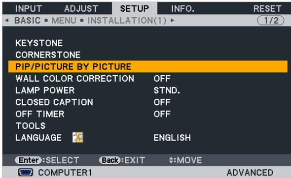
The [PIP/PICTURE BY PICTURE] menu item has the following three options: MODE, POSITION, and PIP/PBP SOURCE.
