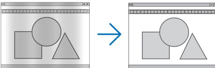
**FREQUENCY** ..... Use this item to fine tune the computer image or to remove any vertical banding that might appear. This function adjusts the clock frequencies that eliminate the horizontal banding in the image. This adjustment may be necessary when you connect your computer for the first time.
