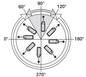
Restrictions for using the projector in ECO MODE at high altitudes:
