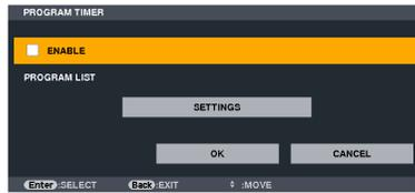
This option turns on/off the projector and changes video signals, and selects ECO mode automatically at a specified time.
