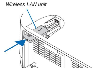
**NOTE:** If the wireless LAN unit is hard to insert, do not push it in by force.
