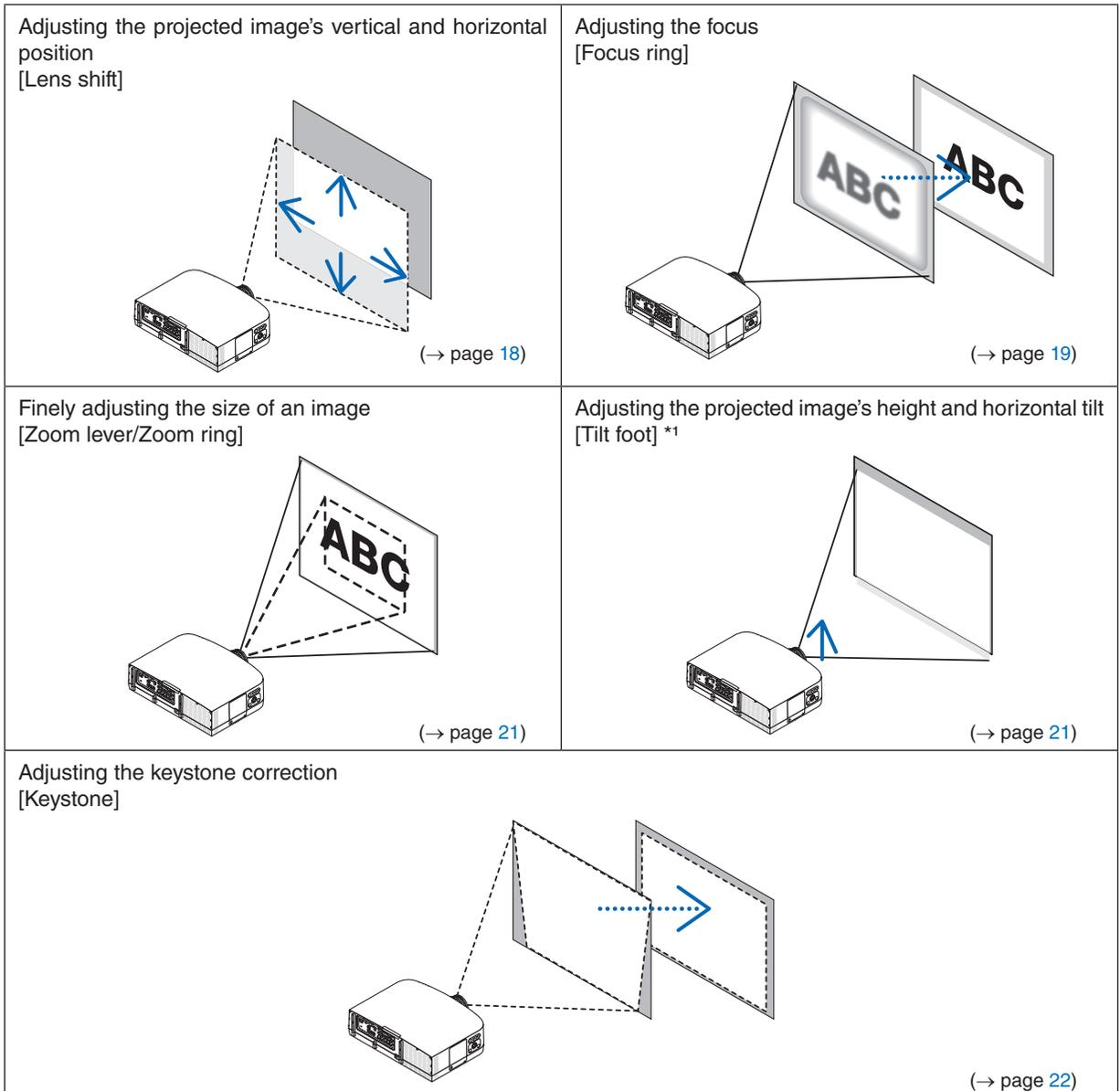
**NOTE\*1:** Adjust the projected image's height using the tilt feet when you want to project the image at a position higher than the lens shift adjustment range.
