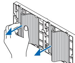
(2) Push the left edges of the filters and remove the two hard honeycomb filters.
