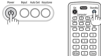
2. Secondly, press the Enter button or press the
