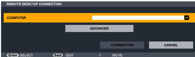
4. Operate the wireless keyboard to input the IP address of Windows 7 and click “CONNECTION”.
