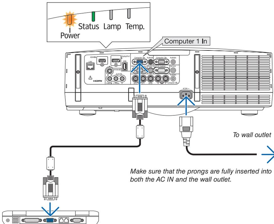
Make sure that the prongs are fully inserted into both the AC IN and the wall outlet.
