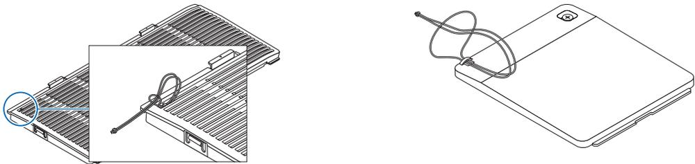
2. Insert the knot in the strap into the hole on the bottom of the projector and pull in the direction of the arrow to fasten.
