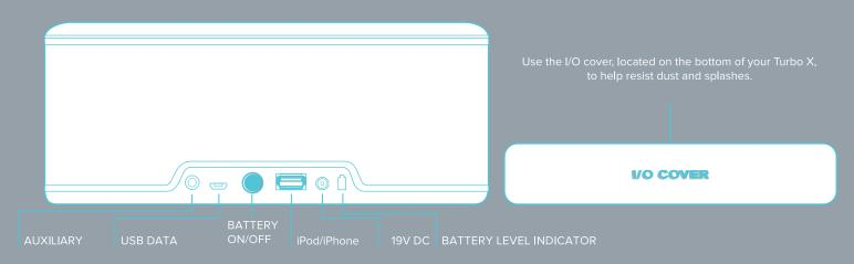
NOTE: Do not cover or stick anything into the input openings (paper clips, nails, gum, etc.) except the I/O Cover or appropriate plugs. Doing so will void your warranty
