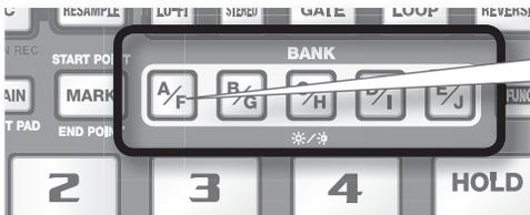
Use the [A/F]–[E/J] buttons to switch the sample bank. To select bank F, Press the [A/F] button twice so it starts blinking.
