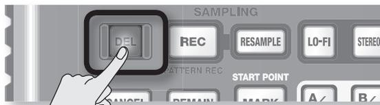
2. The display will indicate "dEL," and the pads that can be deleted will blink.
