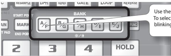
Use the [A/F]–[E/J] buttons to switch pattern banks. To select F, Press the [A/F] button twice so it starts blinking.
