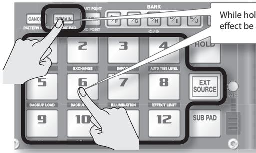
While holding down [REMAIN] button, press the desired pads to have the effect be applied to each pad that is lit.
