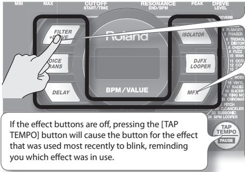
Use these buttons to switch effects (to switch an effect off, get the button's light to go out). You can't apply multiple effects simultaneously.
