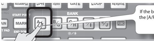
If the button is blinking, bank F is selected. Press the [A/F] button once again so it lights steadily.
