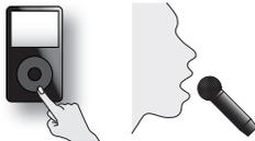
**6-2.** Adjust the volume of the device (e.g., portable music player) connected to the SP-404SX so that the PEAK indicator lights occasionally.
