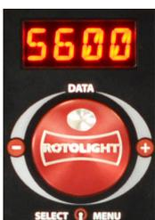
ANOVA's menu can be accessed via the encoder knob on the backplate. Rotating the knob will toggle through the menu items, press the encoder knob inwards to make a selection.
