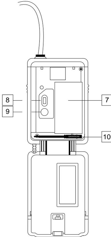
**8: Power on-off switch\*** - Use this to turn the UT1L / UT1G on or off (to conserve battery power, be sure to leave it off when not in use).
