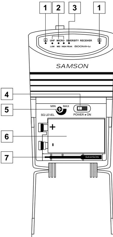
**1: A/B Receiver LEDs** - When signal is being received, one of these will be lit orange, showing you whether the (left) "A" or (right) "B" receiver is currently being used. The UM1 constantly scans its two antennas and automatically selects whichever is receiving the strongest, clearest signal. This *True Diversity* switching is completely inaudible, but it effectively increases overall range while virtually eliminating potential interference and phase cancellation problems.
