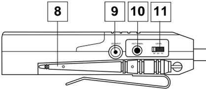
**9: DC input** - This jack will accept a DC input voltage of 6 - 13 volts (inner connection [tip] positive, outer connection [sleeve] ground) from your video camera, if available. Connect the optional Samson AC300R adapter here to charge a rechargeable 9-volt Ni-Cad battery.
