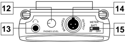
**12: Level control** - This knob sets the level of the audio signal being sent to the headphones output (see #13 below).
