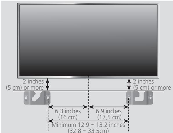
1. Place the "Wall Mount L" on the desired wall surface while paralleled to the floor as shown above, and fix a screw through the hole on its right end.
