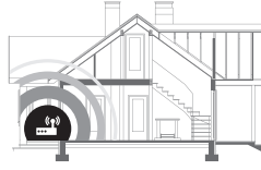
Unsuitable router position
