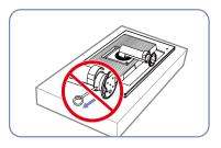
Do not remove the fixing pin until Insert the stand base into the you are finished attaching the stand.
