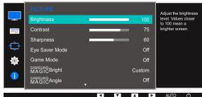
4 Adjust the Brightness using the [▲/▼] buttons.
