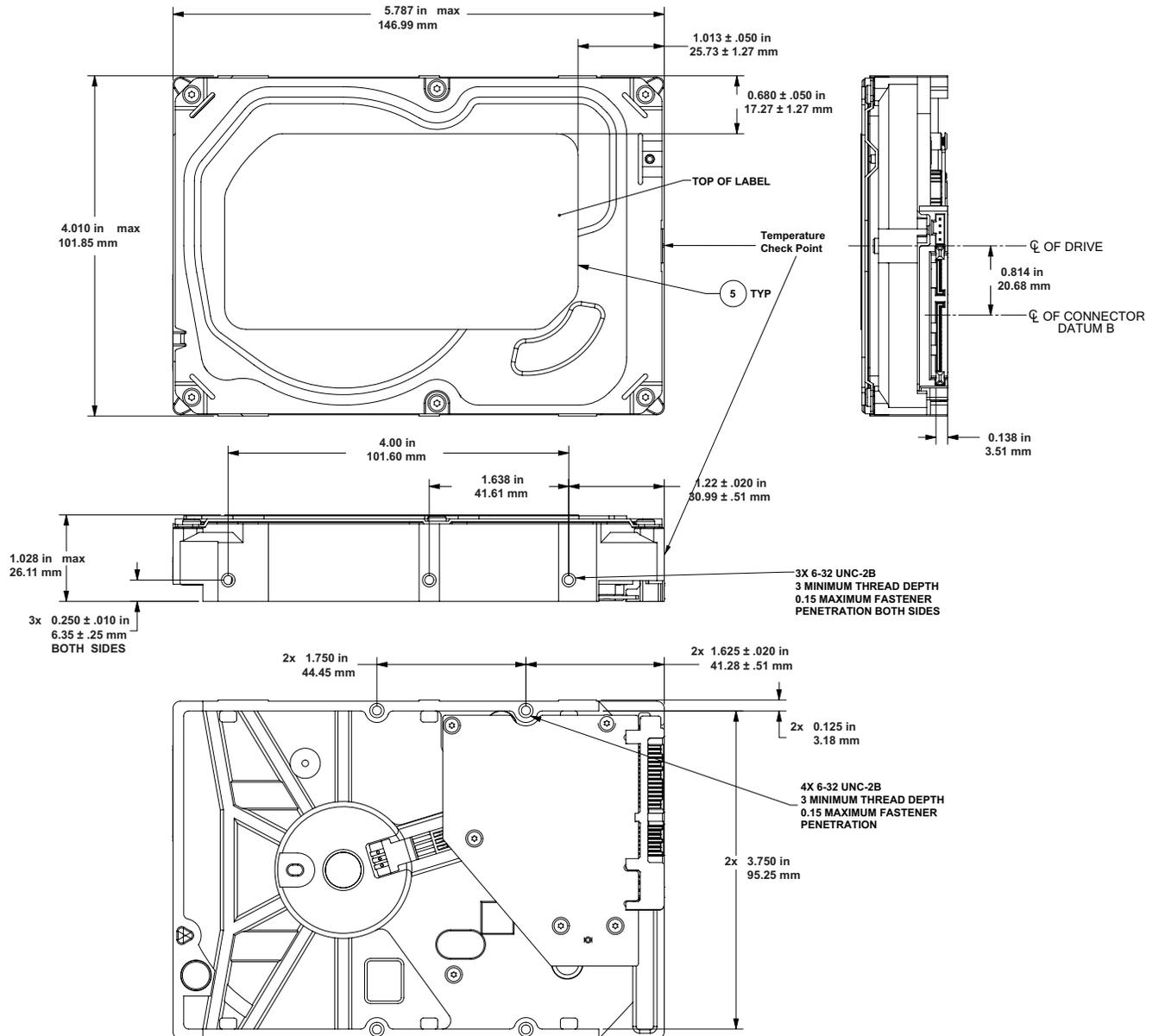
**Note** Drawings are for mounting hole reference only. PCBA show in pictorial only and can vary based on specific customer configurations.
