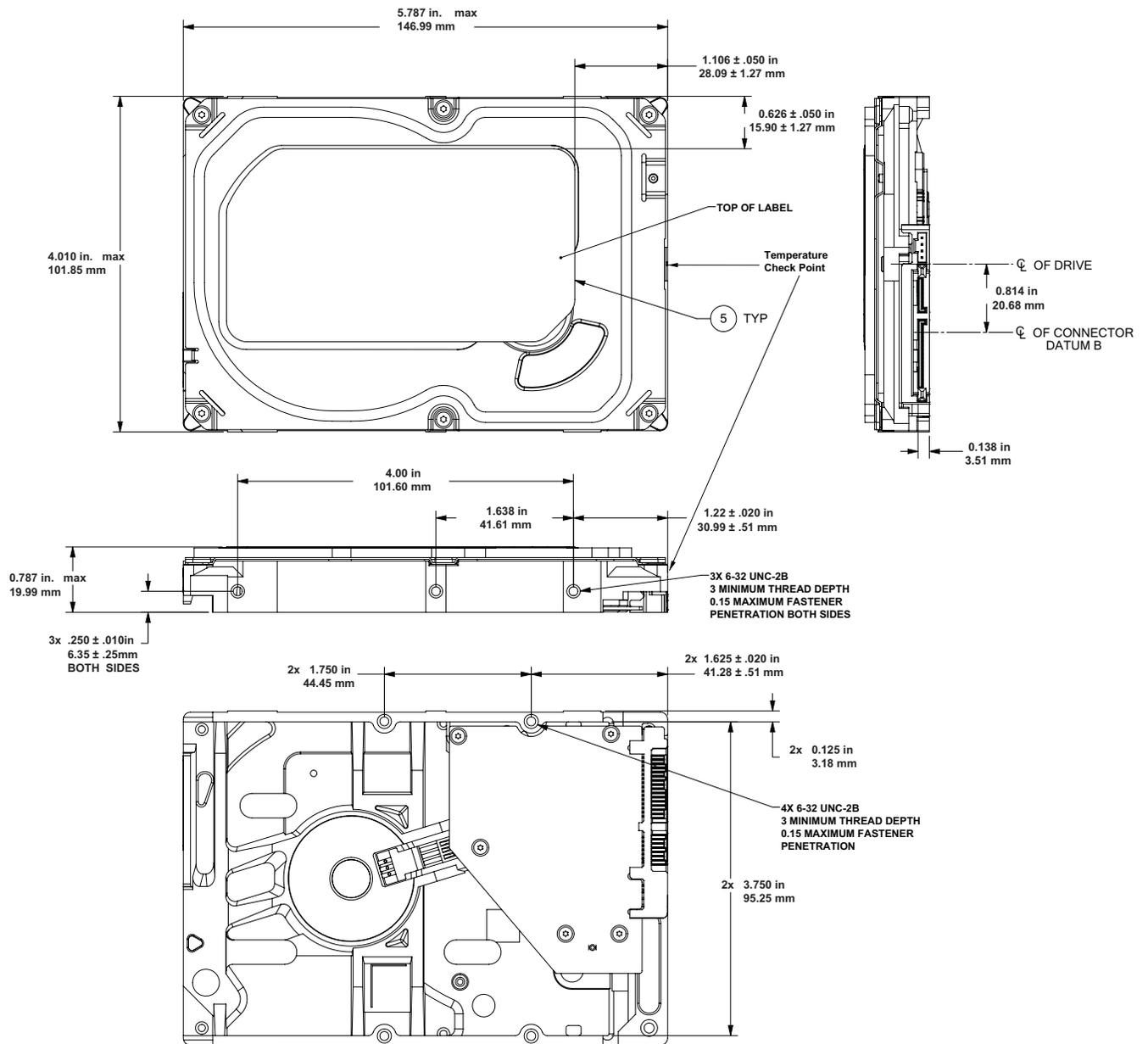
**Note** Drawings are for mounting hole reference only. PCBAs show in pictorial only and can vary based on specific customer configurations.
